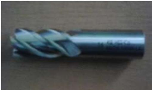
Gambar 3. Cutter Endmill HSS
