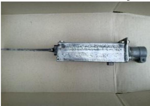
Gambar 6. Alat Panen Sawit Mekanik Bagian Samping
