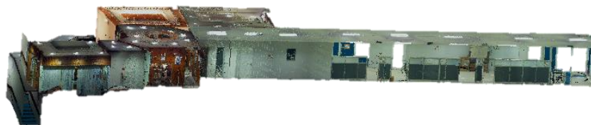
Gambar 3. Tampilan model hasil pengukuran Terrestrial Laser Scanner .
