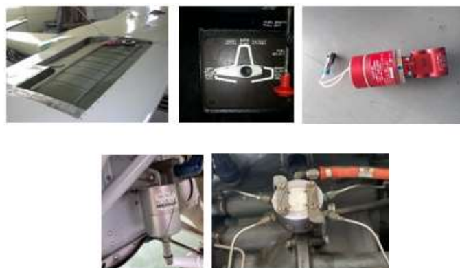
Gambar 2. (A) Fuel Tank , (B) Selector Valve , (C) Fuel Pump , (D) Fuel Filter , (E) Fuel Distributor ).
