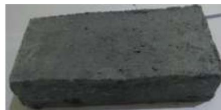
Gambar 2. *Paving block* Berbahan Baku Abu Boiler.
