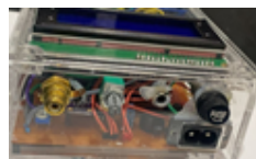
Gambar 5. Input Sinyal Suara, Tuning Control , Output Amplifier, Fuse, Input Kabel Power.
